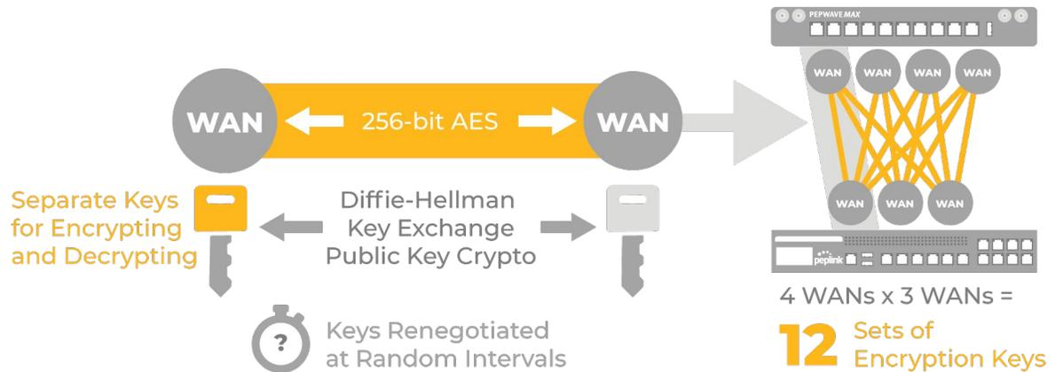
Once the bandwidth bonded SpeedFusion tunnel is formed, sessions are broken down and the resulting packets are sent separately across as available WAN-to-WAN connections. Because each WAN-to-WAN connection is encrypted separately, potential hackers would need to obtain the key to every WAN-to-WAN connection before they stand a chance of accessing the data contained within. This makes SpeedFusion SD-WAN technology virtually impervious to man-in-the-middle attacks.
