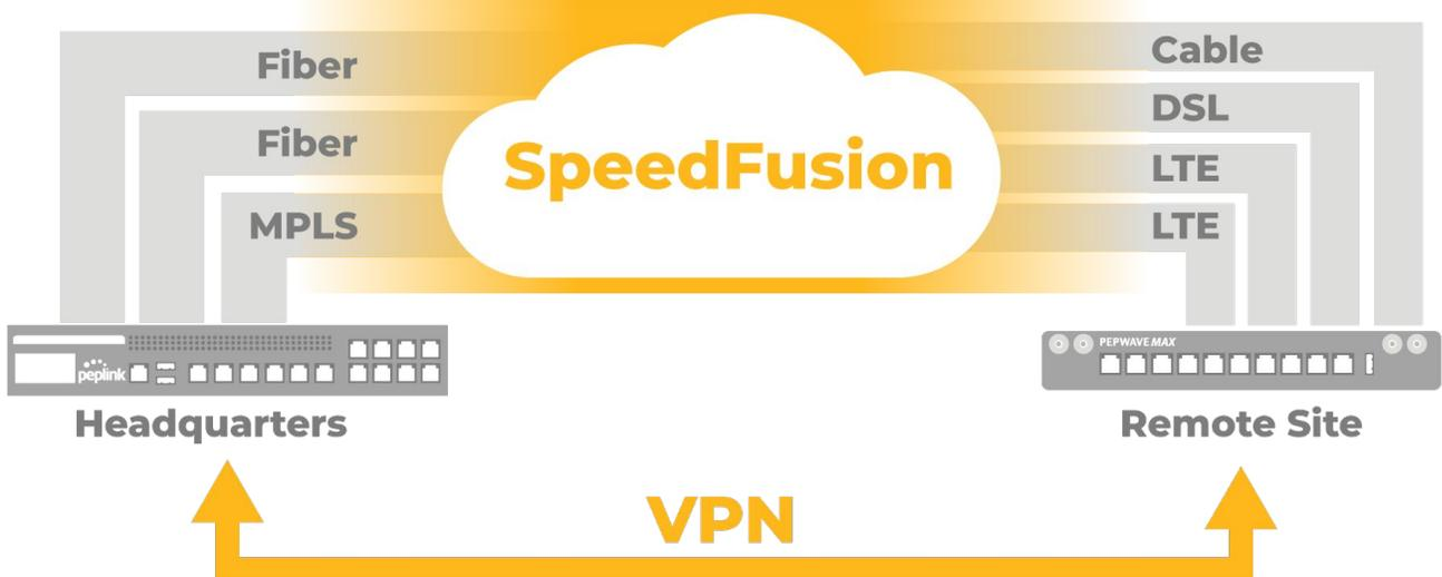
One of SpeedFusion's most powerful features is that it can use multiple WAN links to create a single logical VPN tunnel between devices. This allows SpeedFusion bonding to provide two key functions: bandwidth aggregation and VPN reliability.
